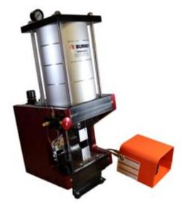
BURNDY® introduces the new OEM840NCP pneumatic press to its line of OEM tooling products. The OEM840NCP bench top pneumatic press is fast, reliable and produces a high quality crimp every time. With its many safety features and high speed pneumatic crimping, it is the perfect tool for a busy production line.
